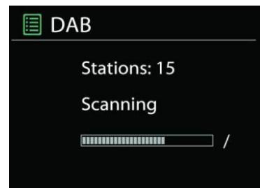
To start a scan manually, choose Full scan. To scan only stations with good signal strength, select Local scan.
