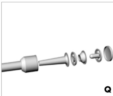
side of the worm with the plastic end has to face the worm housing when putting it inside the worm housing. If the worm is correctly assembled when the plastic end of the worm stands a few millimetres out of the worm housing. Take the adaptor disc. The small end with the recess has to face the worm when attaching. If necessary turn the adaptor disc a little bit until the arresting pin of the worm housing locks precisely into the corresponding recesses of the adaptor disc.
