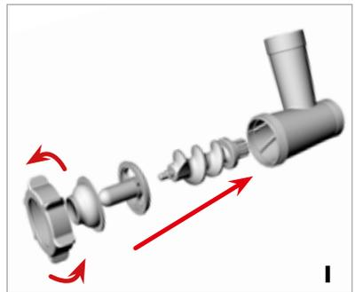
and the axis of the worm stands out 2 mm of the grinding disc.
